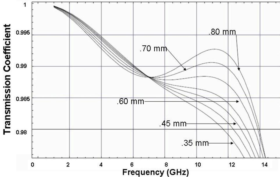
Figure 5: Glass and Teflon transmission with different Teflon thicknesses
