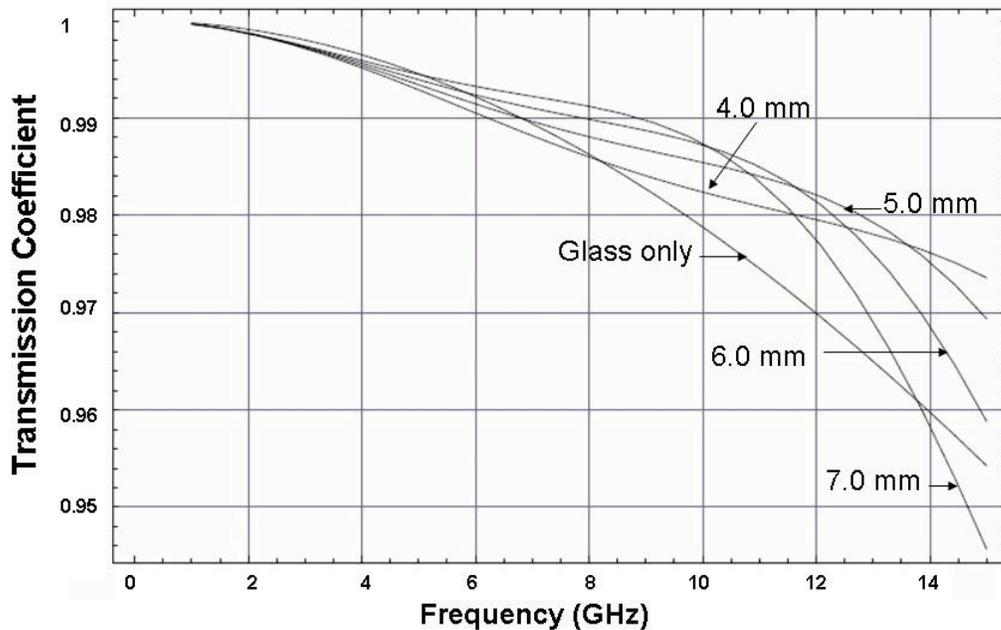
Figure 4. Transmission through the .51 mm glass and Teflon
