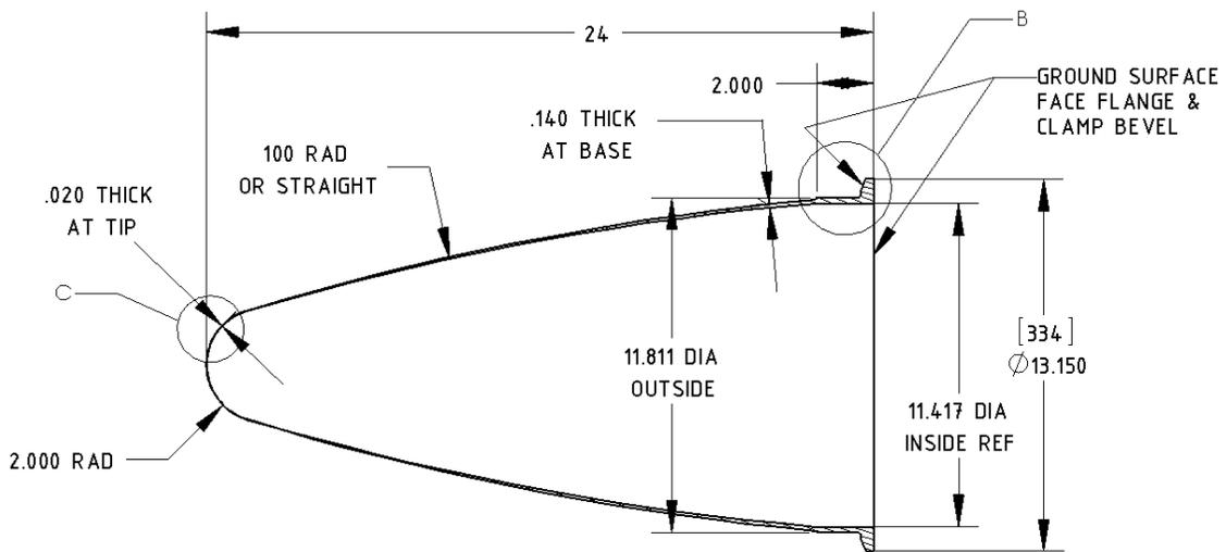
Figure 2. Section view of the glass dome.
