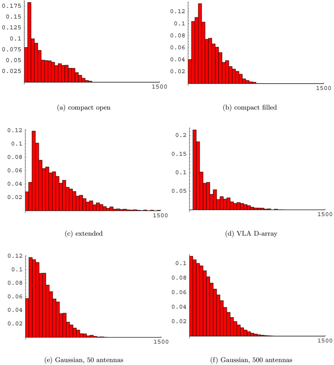
Fig. 3.— Histograms of  $u-v$  density for the three sample configurations, and for comparison, for three additional arrays (see text). The x-axis scale is in meters, while the y-axis scale shows the proportion of visibilities in each bin.
