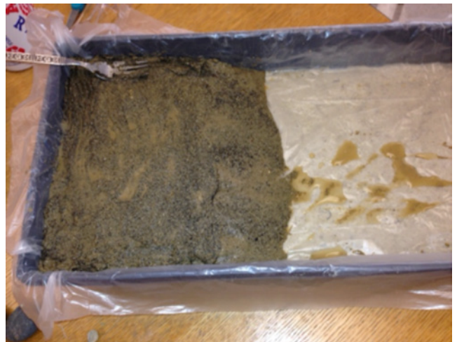
Prop up the sand-filled end 10 degrees with foam slices.
