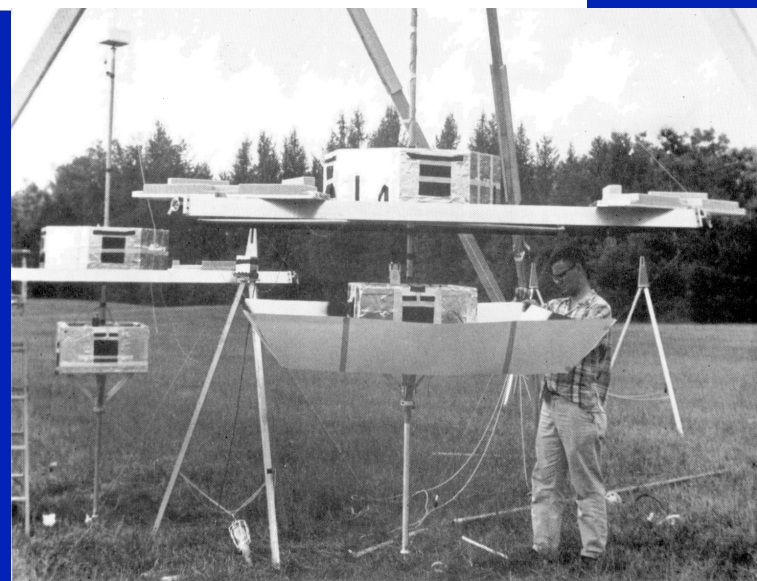
FIG. 2.—The two balloon gondolas. The upper horizontal band occulted the inner part of the corona for the cameras in the lower box. The lower light shields prevented bright light from the lower atmosphere from striking the lenses of the lower cameras.
