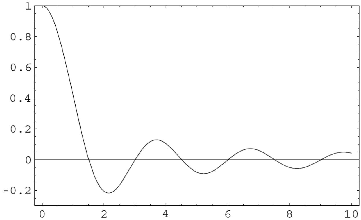
Figure 2. The correlation length  $C(d)$  of the 100 MHz bandwidth signal as a function of extra distance  $d$  in meters that a multipath signal would travel.
